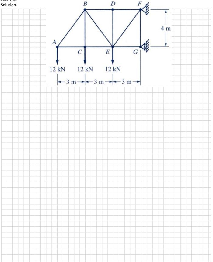
4-20 Refer to Fig. P4-20. Determine the forces in members AC, CD, and DF of the truss due to the loading shown. Solution.
